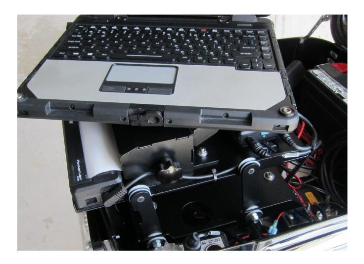
The FMS Accessories articulated mounting base is designed to attach directly to the threaded stand-off's inside a standard Harley-Davidson radio box. There are four pre-drilled holes in the base plate that should line-up with those four stand-off's inside the radio box. Use the same  $\frac{1}{4}$ " x 20 TPI bolts that attached the cover plate inside the radio box.
