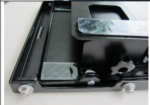
Note: The Whelen top case requires adapter brackets to lower the floor height to provide enough room for the assembly. Remove the stock floor plate and stand-off's coupler nuts.
