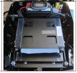
The Brother PocketJet printer attaches using the Velcro strips provided. Note that the RH articulating arm is undercut to provide clearance for the printer power plug. Ensure that the power plug cable is routed carefully to enable the printer paper door to be removed at some point.
